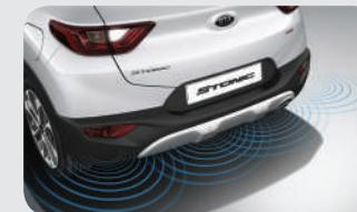
**Parking Distance Warning-Reverse (PDW-R)** When you back into a parking spot, audible beeps alert you to the distance to obstacles behind as you reverse.
