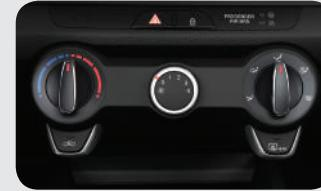
**Manual A/C** The manual air conditioning includes dials for temperature, fan speed and airflow points, with more buttons for modes, defrosting and recirculation.
