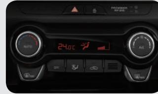
**Auto Temperature Control** Auto temperature control lets you select a desired temperature for the system to maintain. A digital readout displays temperature and settings.
