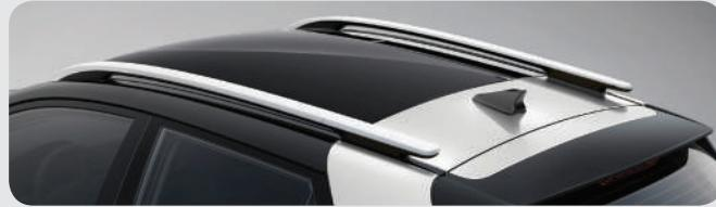
**Bridge-type roof rack** Store bikes, luggage or bulky sporting goods securely on the roof to preserve interior space and protect the upholstery from soil and moisture.
