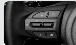
**Steering wheel audio remote** Adjust audio settings using just your thumb for enhanced driving safety.
