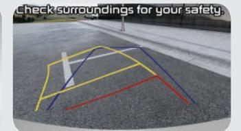
**Rear view camera with dynamic guideline** The rear view camera projects dynamic, bending guidelines onto the image in the 7-inch dash display to recommend a path.
