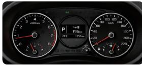
2.6-inch mono-LCD Get tire pressure alerts and other essential vehicle and trip information at a glance with the mono LCD located between the instrument dials.
