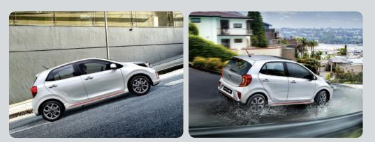
HAC (Hill-start Assist Control) At a standstill on an ESC (Electronic Stability Control) ESC ensures optimal inline, HAC prevents you from rolling backward by gently braking performance and directional control by applying the brakes, for up to two seconds, from the automatically delivering the right amount of braking time you lift your foot from the brake pedal, giving you force to each wheel based on engine torque and driving time to switch your foot smoothly to the accelerator. circumstances.
